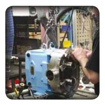
After final assembly, a Waukesha Universal remanufactured pump is performance tested and granted a full factory warranty. You get the same quality and reliability of a new pump at substantial savings in cost.
