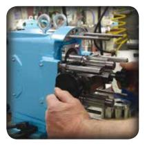
Pump wear is unpredictable. Pitting, grooves and erosion wear is carefully machined to standard oversized dimensions by experienced technicians using precision equipment.
